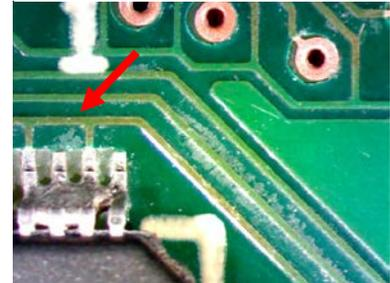
Figure 4: Board cleaned with brush attachment (no separate aerosol was used). No pre-rinse or final rinse utilized. White residue shown around QFN B and QFP, respectively.
