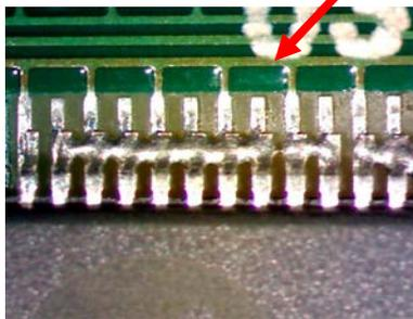
Figure 5: Board cleaned with brush attachment (separate aerosol was used for pre-rinse and final rinse). Some white residue shown around QFN B and QFP, respectively.
