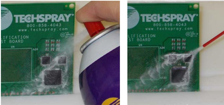
Figure 1: Visual comparison of an aerosol spray without (left) and with a straw attachment.
