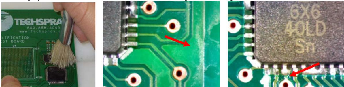
Figure 2: Board cleaned with handheld brush. The components were wetted, and then the brush was wetted and used to scrub the contaminated area. The board in the first picture did not undergo a final rinse. The board in the second picture did (Note: all flux was not removed).
