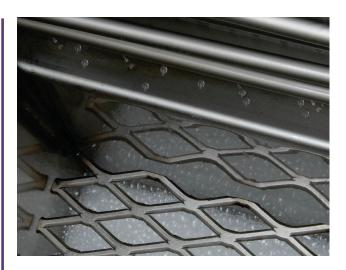
4. Use the retained solvent (from step 1) to refill the vapor-degreaser and add whatever volume of solvent is necessary to completely fill the machine.
